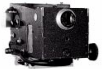
The 'Shoebox' Gunsight Anti-aircraft guns of 1939 couldn't cope with fast flying planes. Draper displaced the fixed sight of the gun by placing the computing 'shoebox' directly on the gun, enabling the gunner to hold the reticle on a moving target.
